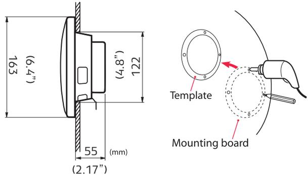
2. Use the template supplied to mark the position of the mounting screws and the outline of the speaker hole. Drill the mounting holes using a 3.3 mm drill bit and cut the hole for the speaker.
