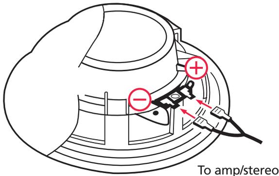
2. Remove the speaker grille (turn anti-clockwise). Fit the speaker into the cutout and secure the speaker using the screws (supplied).
