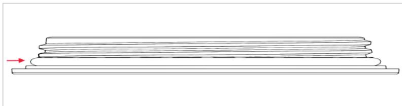
11. Ensure lid is closed correctly and is tightened to the correct torque. The O-Ring should not be visible when correctly tightened.
